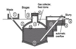
Figure 2. Biodigester fixed dome type
